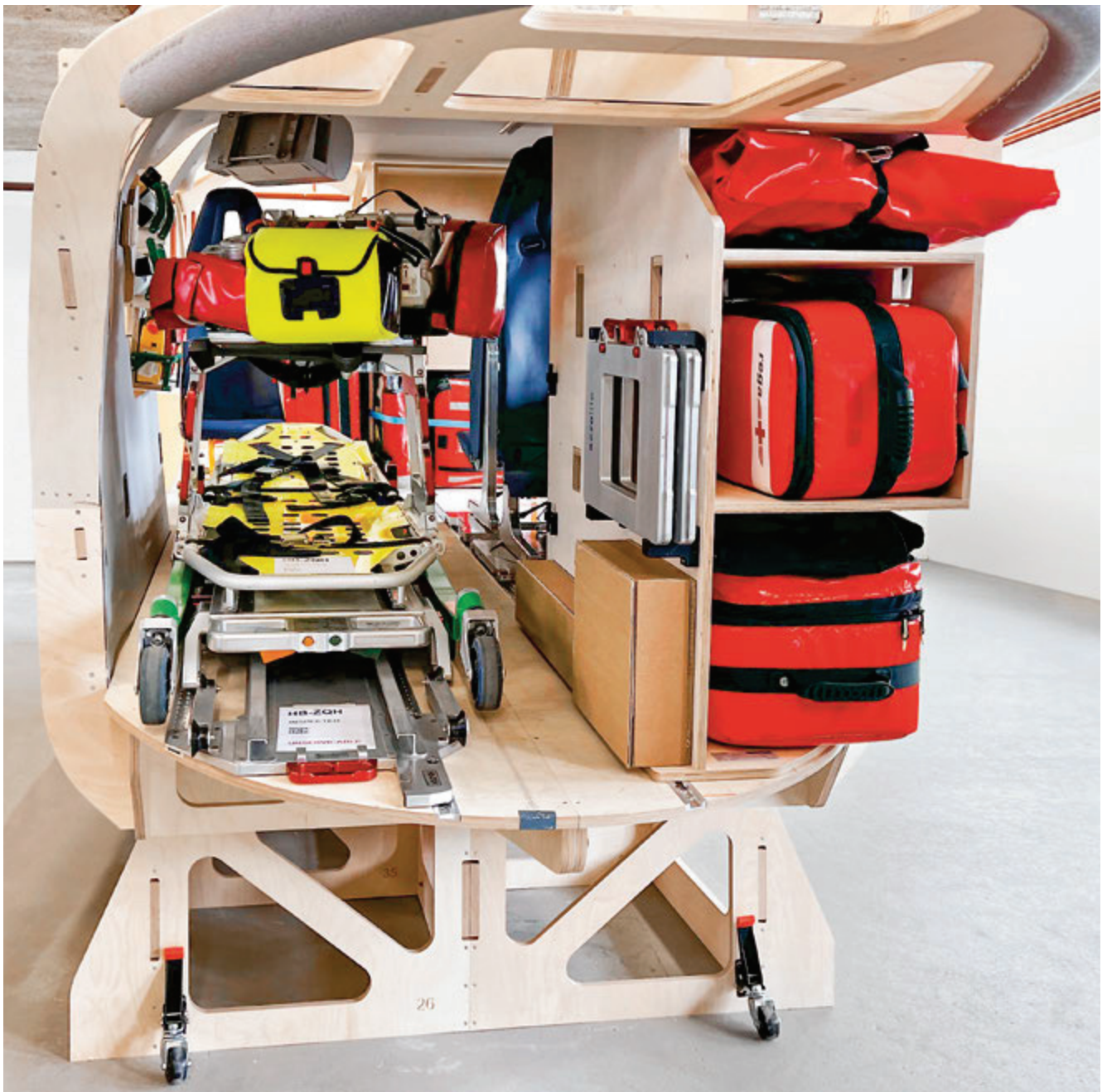
A full-scale wooden model was built to enable adjustments to be made in the cabin.
