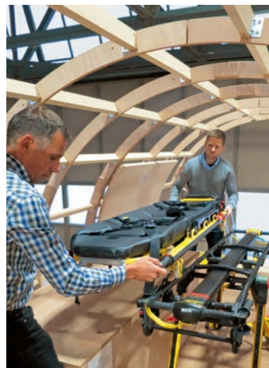
Test in the mock-up of the Challenger 650: do the stretcher systems from the ground ambulances also fit on the wider intensive care units in the new Rega jet?
